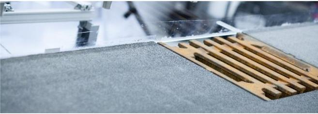
Investigate different influencing parameters such as longitudinal and transverse slope, grate geometry or discharge.
